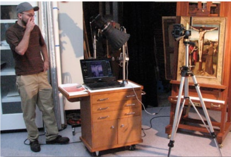
Carlos Moya, conservation intern at the Chrysler Museum of Art, demonstrated the use of the lab's new Fujifilm IS Pro UV-IR camera. The camera and imaging software, originally developed for use in criminal forensic labs, is an extremely useful tool for examining art objects with specific wavelengths of light. Here, Carlos is conducting infrared examination of "Christ on the Cross", attributed to Gerard David.
