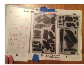
Mylar template used to record the weights of objects as they undergo freezedrying. PowerPoint slide courtesy of Lesley Haines.
